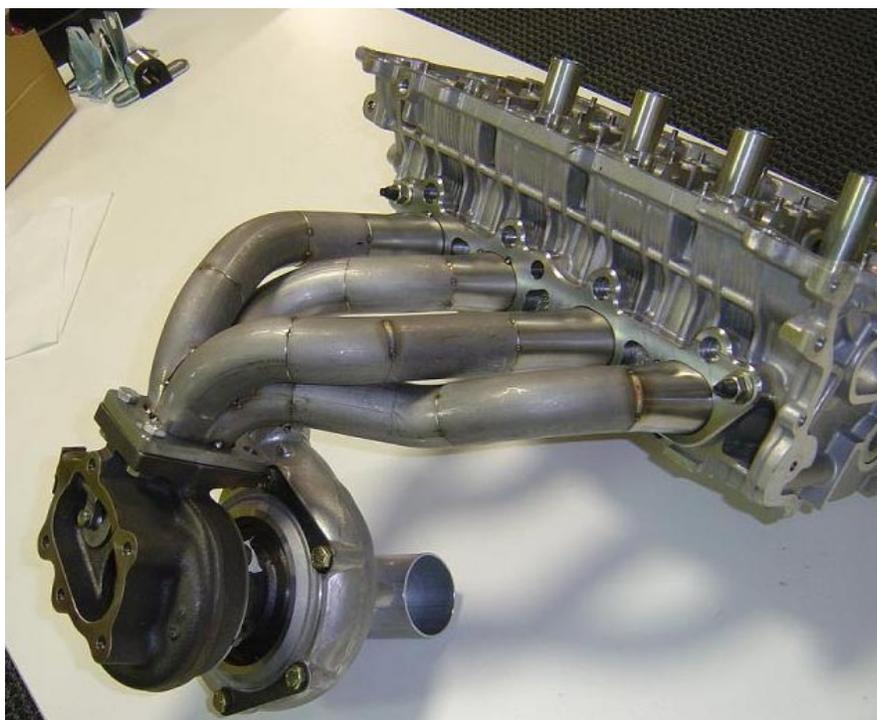
*Exhaust manifold & turbo. Note how the manifold tapers to smaller diameter runners in order to maintain the velocity of the exhaust charge.*
