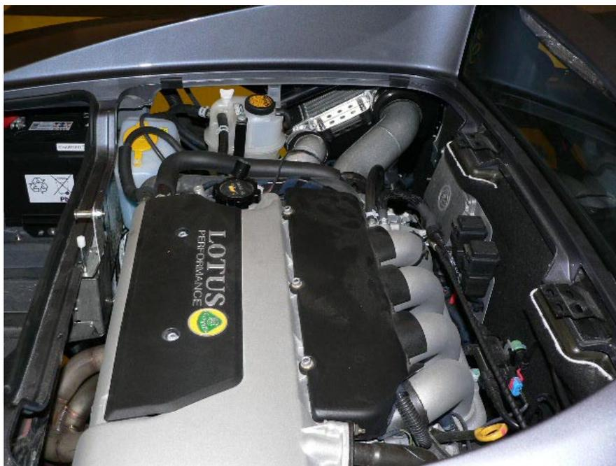
**The intercooler is at the top-right and the exhaust manifold can be seen between the engine and the boot (trunk).**
